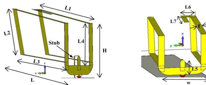
**Figure 1.** Proposed wideband LTE/5G antenna designed to be integrated under shark-fin cover on a vehicle roof. Dimensions:  $H = 35$ ,  $L = 40$ ,  $L1 = 35.8$ ,  $L2 = 29.1$ ,  $L3 = 35$ ,  $L4 = 27$ ,  $L5 = 12$ ,  $L6 = 12.5$ ,  $L7 = 9.65$ ,  $W = 40$ ,  $t = 5$ ; all units are in mm.
