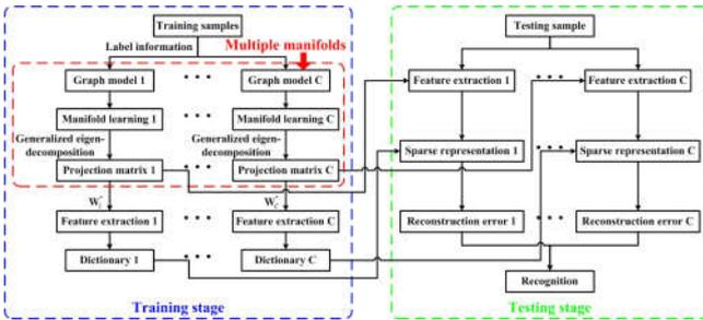
Figure 2. Flow diagram of the proposed MMSR algorithm.
