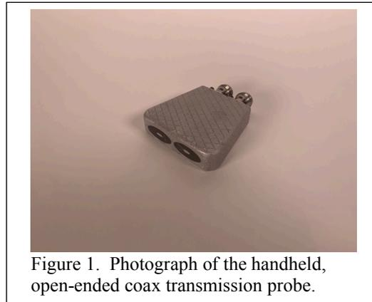
Figure 1. Photograph of the handheld, open-ended coax transmission probe.
