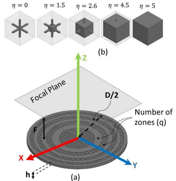
**Figure 1. (a) The geometrical principle of the Fresnel zone plate, (b) Brakora static modeling for the proposed porous cell.**
