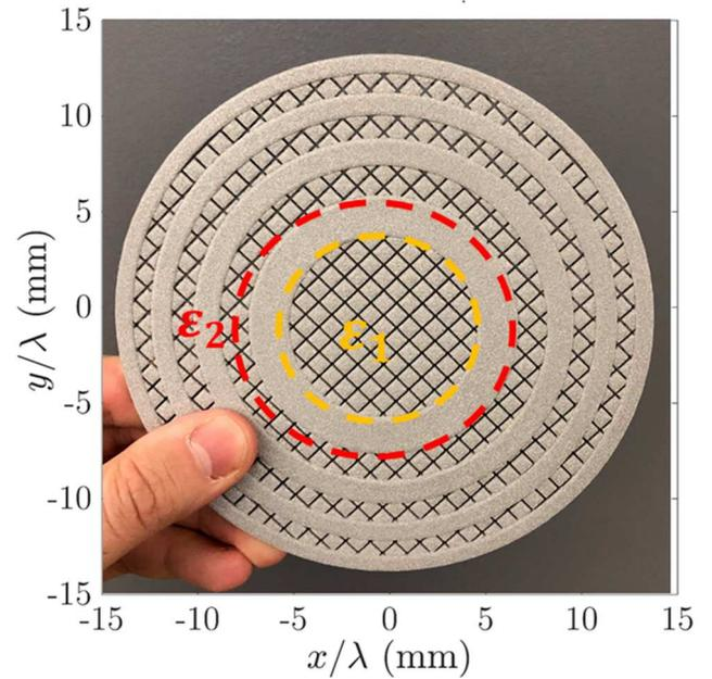
Figure 2. Fabricated alumide based half-wave zone plate.
