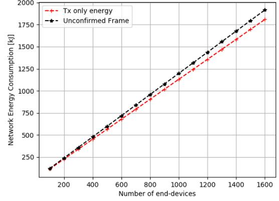
**Figure 3.** Evolution of NEC as a function of the number of nodes for scenario 0 and scenario 1.
