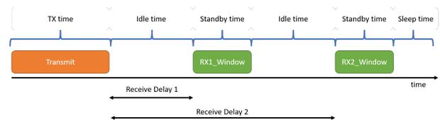
Figure 2. Channel Access for LoRaWAN Class A End-devices.
