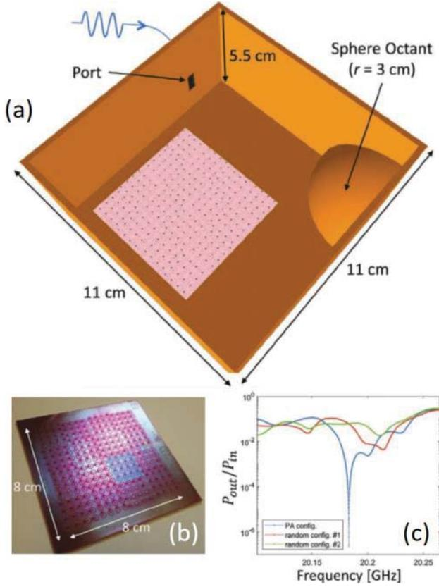
**Figure 1.** (a) Experimental setup involving a disordered 3D chaotic cavity excited by a single channel (coax waveguide). One wall is equipped with a 16-element programmable metasurface. (b) Photographic image of the metasurface. (c) Experimentally measured reflected power for the metasurface configuration yielding PA at 20.18 GHz as well as for two random configurations.
