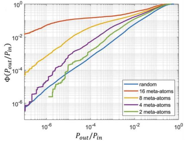
**Figure 2.** Experimentally determined CDF  $\Phi(P_{out}/P_{in})$ . The blue curve is based on the 19 – 24 GHz band and all possible metasurface configurations. The remaining lines consider for each frequency point only the reflected power corresponding to the optimal metasurface configuration, for different numbers of programmable meta-atoms.
