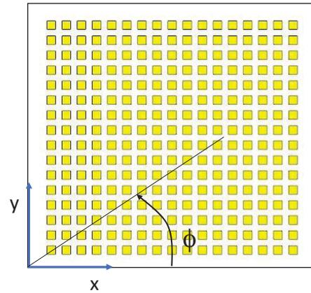
**Figure 1.** Layout of a planar 16 x 16 patch array, on a Rogers RO3003 substrate, for WPT at 24 GHz.
