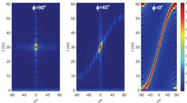
**Figure 2.** Beam-pattern of the patch array of Fig. 1 in the  $\phi=90^\circ$ ,  $45^\circ$ ,  $0^\circ$  planes, when  $f_{0,0}=24$  GHz,  $\Delta f=5$  MHz, and each element of a column of the array shares the same frequency (frequency-diversity is applied to array rows, only).
