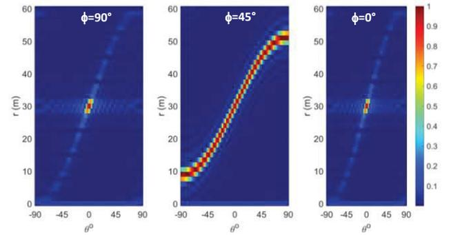
**Figure 3.** Beam-pattern of the patch array of Fig. 1 in the  $\phi=90^\circ$ ,  $45^\circ$ ,  $0^\circ$  planes, when  $f_{0,0}=24$  GHz,  $\Delta f=5$  MHz, and each element of the array has its own frequency (frequency-diversity is applied to both columns and rows of the array).
