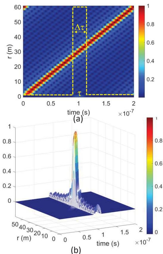
**Figure 4.** Time-control strategy of the FDA of Fig. 1 with frequency-diversity for rows, only. (a) beam-pattern vs. time of a standard FDA with the superposition of the normalized rectangular pulse; (b) 3D beam-pattern when the time control is applied.
