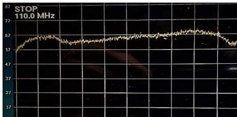
**Figure 4.** Testing the frequency response of the two stage LNA using the Advantest U3751 Spectrum Analyser.
