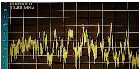
**Figure 5.** Testing free on air HF signals detected utilizing the active dipole antenna and the Advantest U3751 Spectrum Analyser.
