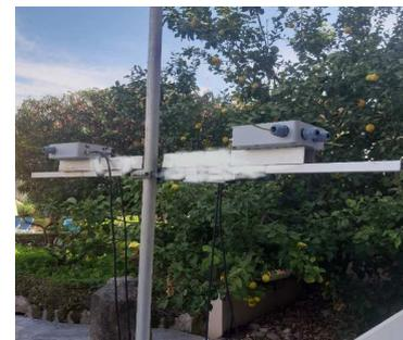
**Figure 7.** The active array under test installed on a temporary mast.
