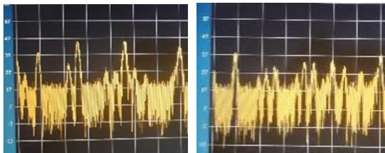
**Figure 8.** Free on air signals before and after rotating the array 180° using the Advantest U3751 Spectrum Analyser.
