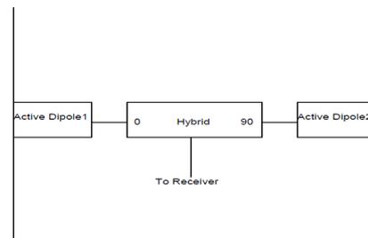
**Figure 3.** The basic sections of the HF active phased array.
