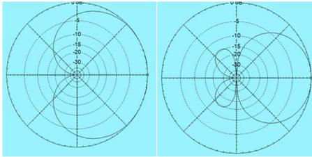
**Figure 3.** The E and H Plane radiation pattern of a  $\lambda/4$  phased array at 10MHz 90<sup>0</sup> phase difference feed simulated using equations (1) and (2).
