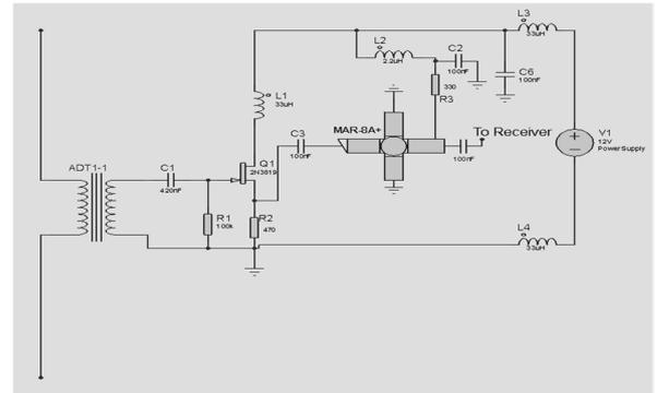
**Figure 2.** The schematic of the two-stage Low Noise Amplifier.
