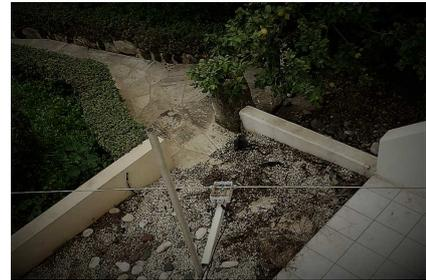
**Figure 6.** The active dipole as a single element.
