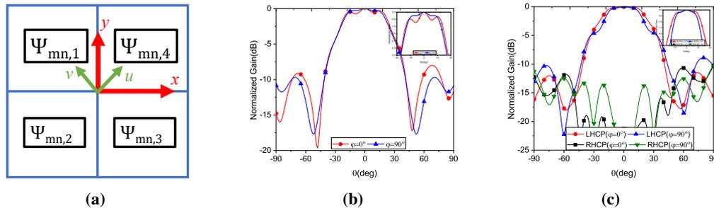
**Figure 1.** Flat-top pattern synthesis with MTS where the antenna is placed in  $-ve$   $z$ -direction: (a) Sub-regions of the MTS, Simulation results at 9.9 GHz, (b) radiation pattern for  $E_x$  incident wave, (c) LHCP and RHCP gain pattern for  $E_u$  incident wave
