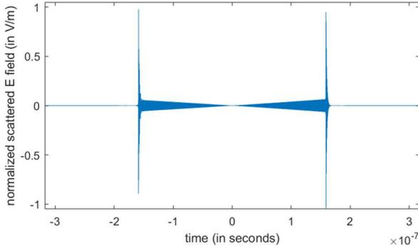
**Figure 4.** The rectangular chirped pulse scattered signal with scattering cancellation implemented, for no delay in the circuit.
