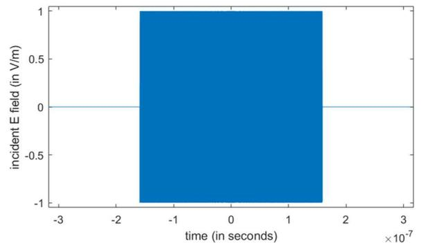
Figure 3. The incident rectangular chirped pulse signal.
