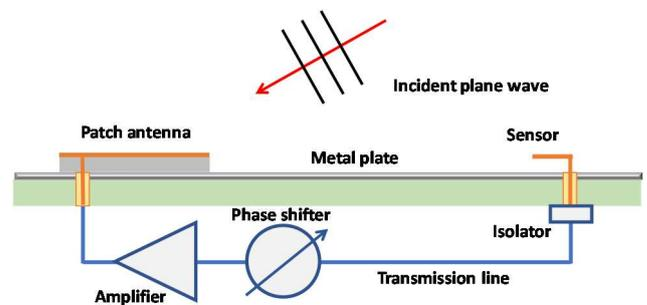
**Figure 2** Geometry of a patch on an object (metal plate), connected by a transmission line to a sensor via an isolator, amplifier and phase shifter.
