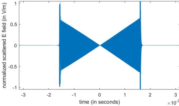
**Figure 5.** The rectangular chirped pulse scattered signal with scattering cancellation implemented, for five wavelengths delay in the circuit.
