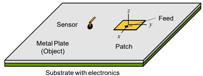
**Figure 1.** The layout of the patch antenna and sensor on an object, with the object taken to be a metal plate for simplicity. The electronics is shown in Figure 2.
