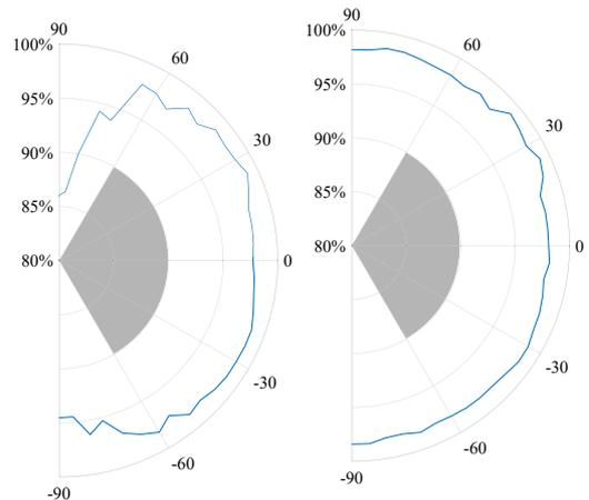
**Figure 4.** Measured system fidelity factor (SFF) as function of the angle. Left: azimuth plane (XY-plane). Right: elevation plane (YZ-plane). As reference, the SFF > 90% goal is marked in grey.
