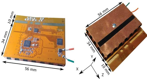
**Figure 2.** Left: final PCB with on the back the cavity-backed slot antenna. Right: cavity-backed slot antenna.
