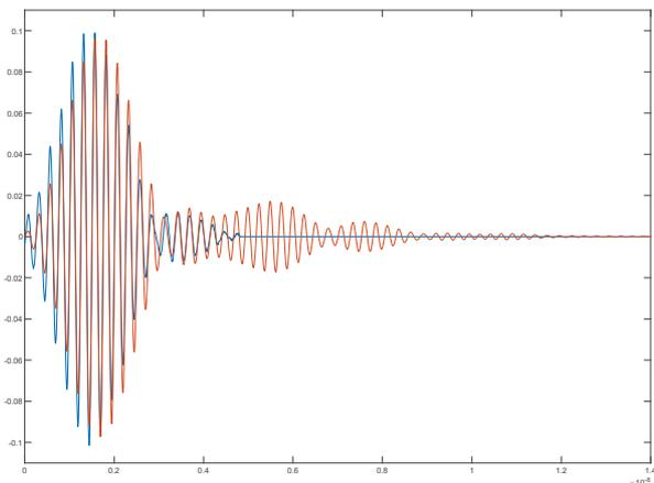
**Figure 3.** Normalised pulse at the transmit antenna (blue) compared with normalised pulse at the receiver antenna (red).
