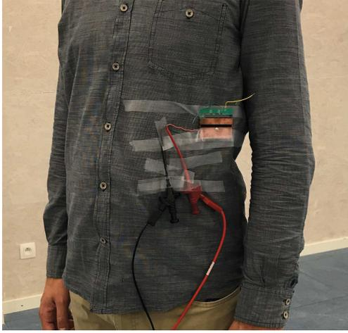
**Figure 6.** Test subject outfitted with the sensor node on the torso, externally powered for measurement purposes.
