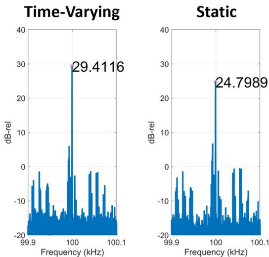
**Figure 4.** Received data from the transmitter operating in time-varying mode with the switch carefully timed (left) and in static mode with the switch kept on (right).
