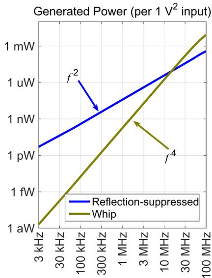
**Figure 2.** Simulated results for radiated power as a function of frequency for both a conventional (green) and a reflection-suppressed (blue) antenna.
