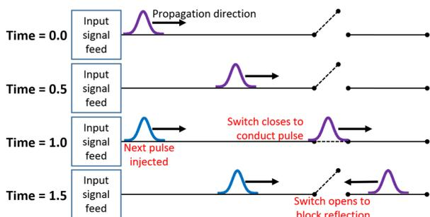
**Figure 1.** A diagram of the time-varying impedance matching technique, with four snapshots in time.
