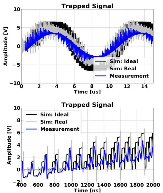
**Figure 3.** Simulated and measured data of trapped pulses from a PAM waveform.
