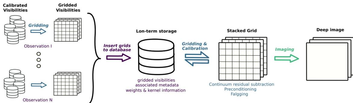
Fig 1.: Deep imaging pipeline: Raw observed data is discarded after the gridding step and only sparse grids and associated metadata are stored in a dedicated database. After the preconditioning is applied the daily grids are stacked together. Further calibration of the stacked and daily grids can be applied. The deep image is formed via deconvolution.
