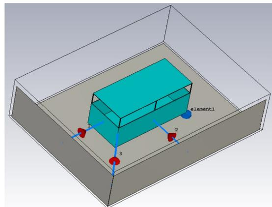
Figure 4. DCI setup with three current sources
