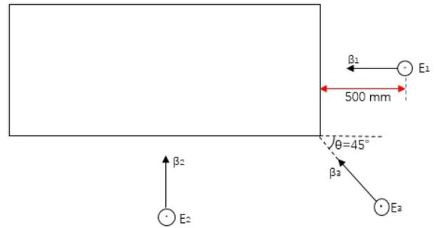
Figure 3. Excitation scenarios for HIRF testing (top view)
