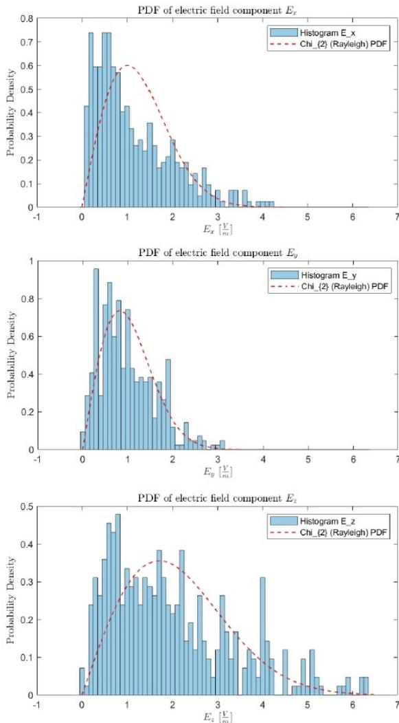
**Figure 5.** Histograms and probability densities for  $E_x, E_y, E_z$  assuming HIRF testing
