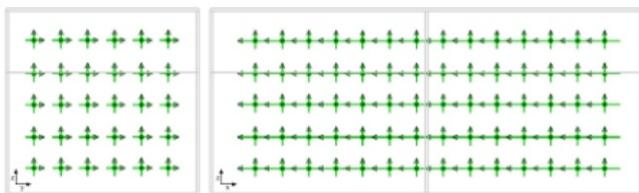
Figure 2. Electric field probes inside the vehicle (left: front view, right: top view)
