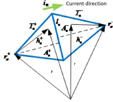
Figure 3. Two-dimensional RWG basis functions
