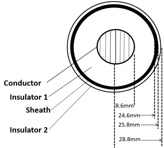
Figure 6. Cross section of high-voltage cable
