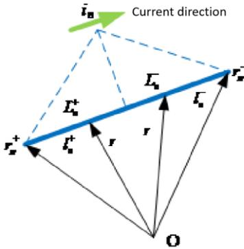
Figure 2. One-dimensional RWG basis functions
