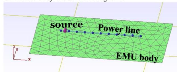
**Figure 1.** Equivalent model for calculating the induced current on the carriage
