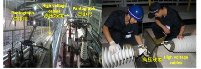
Figure 5. Roof pantograph and cable of CRH2A
