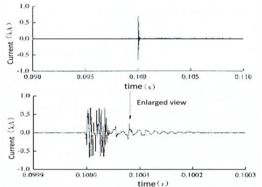
Figure 7. The disturbance current on the high-voltage cable
