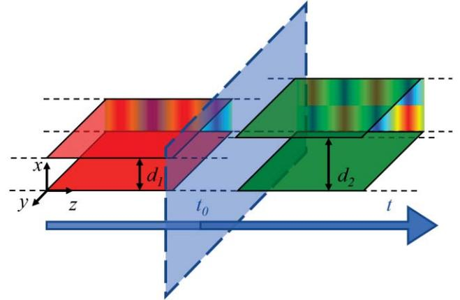
**Figure 1.** Boundary-induced temporal interface in a parallel plate waveguide. The height of the waveguide is suddenly increased from  $d_1$  to  $d_2$  at the time instant  $t_0$ .
