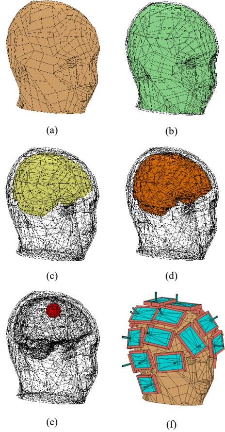
**Figure 2.** Numerical phantom. Outer boundaries of (a) the head phantom made of 3 mm thick ABS layer, (b) head mimicking tissue, (c) 3 mm thick brain layer made of ABS, and (d) the stroke. (e) The antenna array and the phantom.
