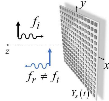
**Figure 1.** A time-varying meta-reflector with surface admittance  $Y_s(t)$ . A plane-wave at frequency  $f_i$  normally impinges the metasurface. A field at different frequency  $f_r$  is reflected back.
