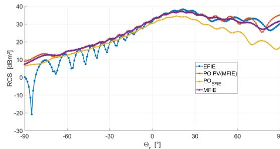
**Figure 2.** Bistatic RCS between  $-90^\circ$  and  $90^\circ$  of the geometry shown in Figure 1, computed with different methods, with  $\Theta_{inc} = -70$
