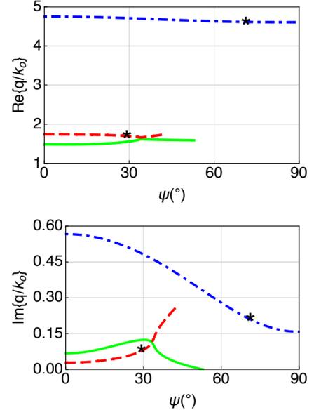
**Figure 2.**  $\text{Re}\{q/k_0\}$  and  $\text{Im}\{q/k_0\}$  plotted versus  $\psi \in (0, 90)^\circ$  for unexceptional (curves) and exceptional (black stars) CPP waves. See text for parameter values.
