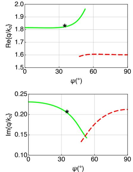
**Figure 1.**  $\text{Re}\{q/k_0\}$  and  $\text{Im}\{q/k_0\}$  plotted versus  $\psi \in (0, 90)^\circ$  for unexceptional (curves) and exceptional (black stars) surface–plasmon–polariton waves. See text for parameter values.
