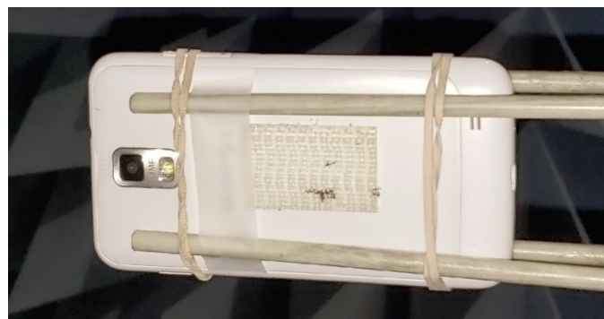
Figure 1. Common mounting schemes for “free-space” mobile phone testing.
