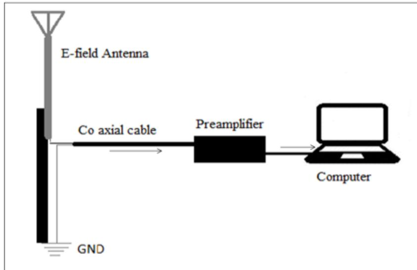
➤ *Schematic diagram of the VLF signal receiving system.*
