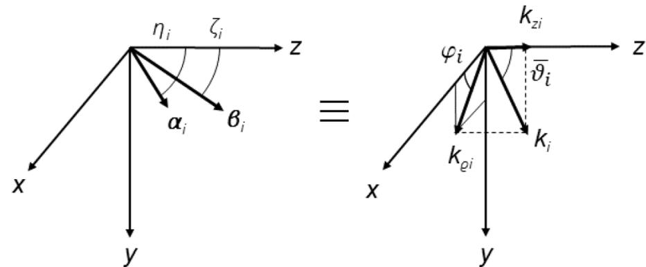
The left figure represents the complex wave vector of an inhomogeneous plane wave with the phase and attenuation vectors. The right figure represents the same vectors with the complex-angle formulation.
