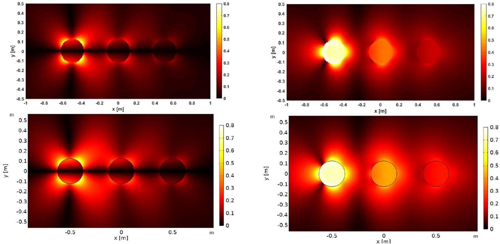
The results obtained with Matlab (top) and Comsol (bottom) in the case of  $k_e = 1-i$  [1/m], for the environment and  $k_c = 2-0.5i$  [1/m] for all cylinders. Right:  $E_x$  component, left  $E_y$
