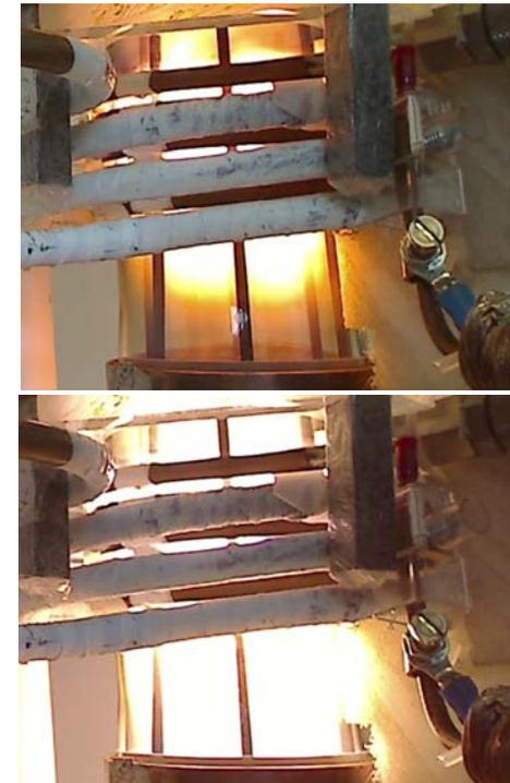
Plasma with total rf power  $P_t=350$  W (above) and 400 W (below); two rf coils and faraday cage partly visible [12]
