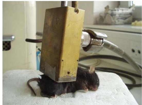
**Figure 1.** Waveguide applicator for biological experiments.
