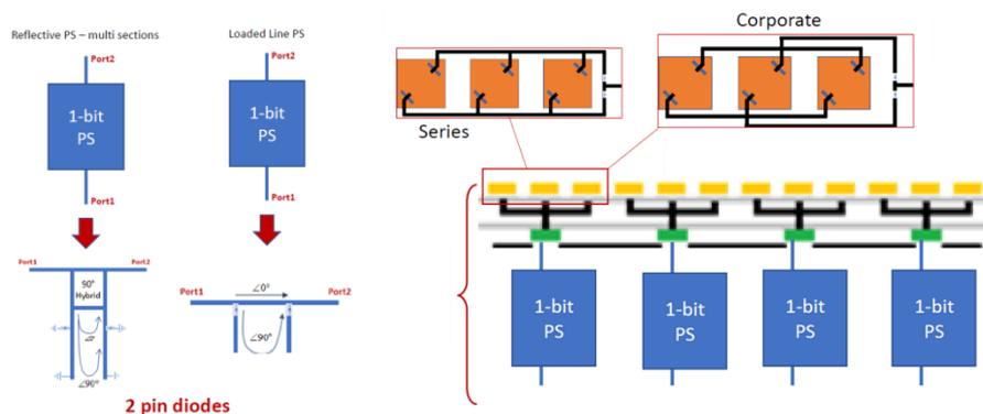
**Figure 1.** Examples of different ways to synthesize the signal phase distribution in portions of a phased array.
