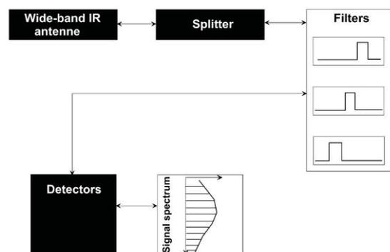
**Figure 1.** Simplified block-scheme of the sensor for measuring the spectrum of incoherent IR radiation.
