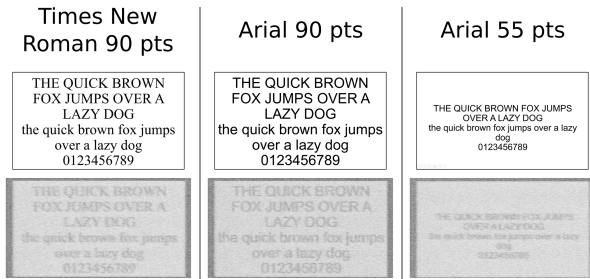
Figure 2. Some examples of the original images and the reconstructed versions. Two fonts, and ten different sizes for each font were used. In each case there were 20 frames for a data set composed of 400 images.
