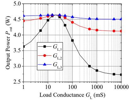
**Figure 4.** Simulated output power  $P_{out}$  as function of varying load conductance for the analysed numerical example. One of the three load conductances is varied, while keeping the other two fixed at their optimal value.
