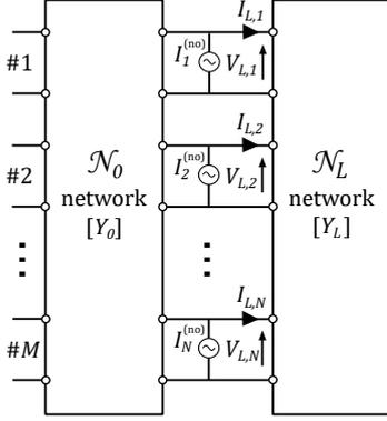
**Figure 2.** Norton equivalent circuit with load network  $\mathcal{N}_L$ .
