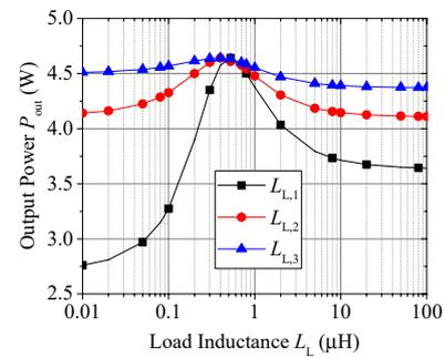
**Figure 5.** Simulated output power  $P_{out}$  as function of varying load inductance for the analysed numerical example. One of the three load inductances is varied, while keeping the other two fixed at their optimal value.
