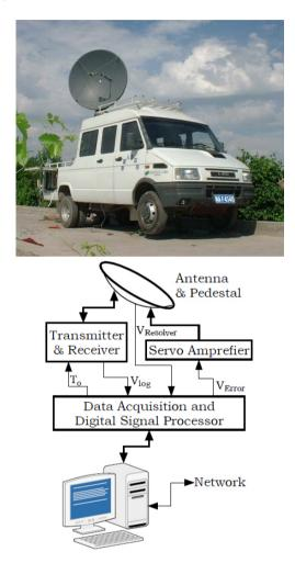
Figure 1. XDR radar system. Up is vehicle borne mobile radar, down is XDR block diagram.
