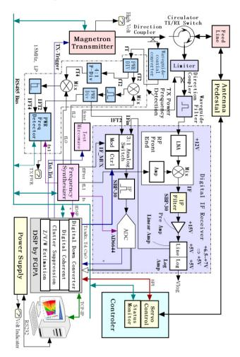
**Figure 3.** WXR-MD-10 Block Diagram (Note that the DDC-Digital Down Converter in Digital IF Receiver is put on DSP-Digital Signal Processor).
