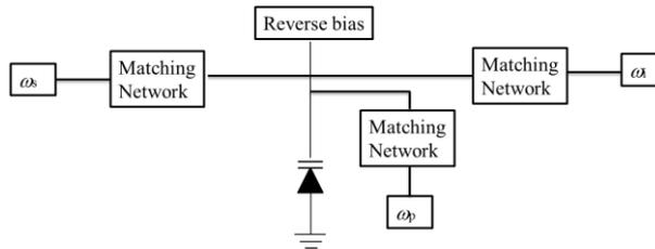
**Figure 1.** Diagram of the proposed varactor-based frequency downconverter.
