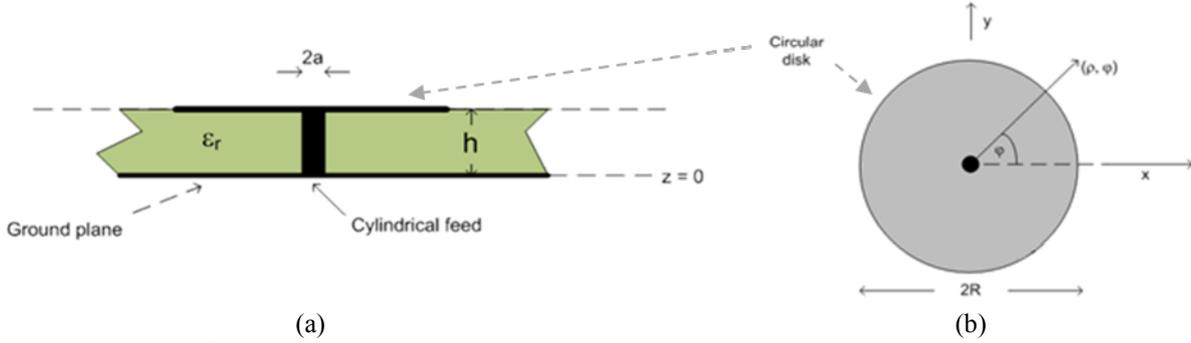
Fig. 1: The center-fed microstrip disk antenna. (a) Side view. (b) Upper view.
