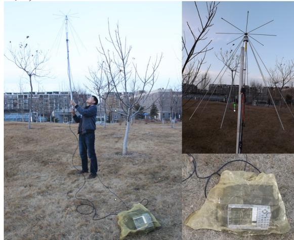
Fig.2 Portable survey Equipments (left): disk-cone antenna and LNA(upper right) and spectrometer (lower right )
