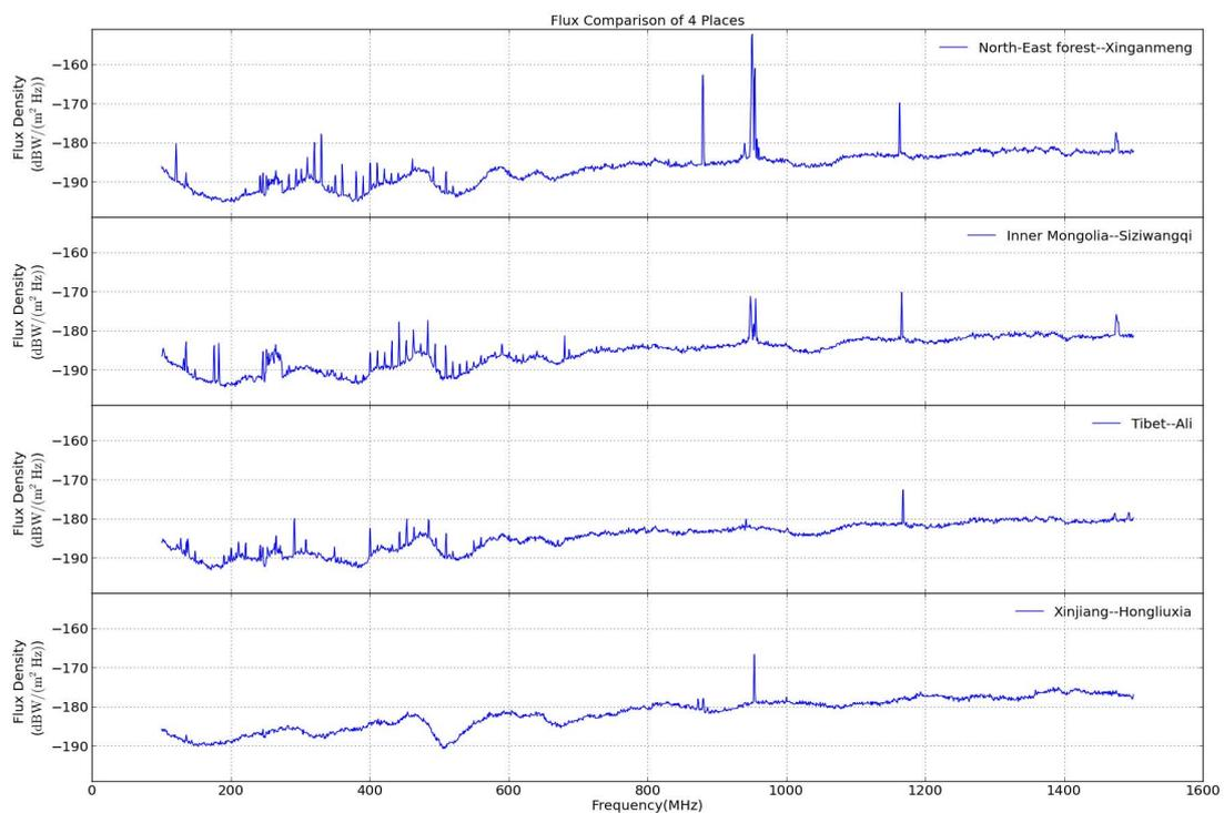
Fig.3. Comparison of RFI spectrum at four sites we survey
