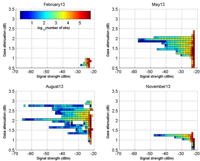
Figure 2. Joint histograms for gaseous attenuation (dB) and the Eband signal strength (dB) for 4 months in 2013.
