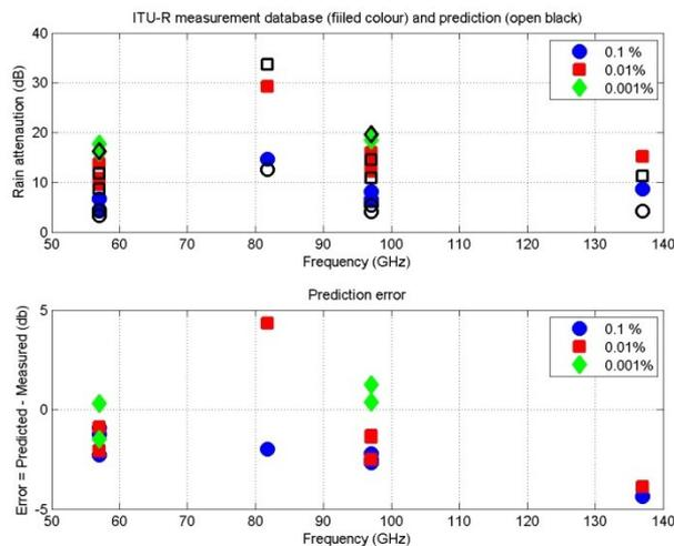
Figure 4. Predicted and measured rain attenuation for links at and above 57 GHz in the ITU-R data base.
