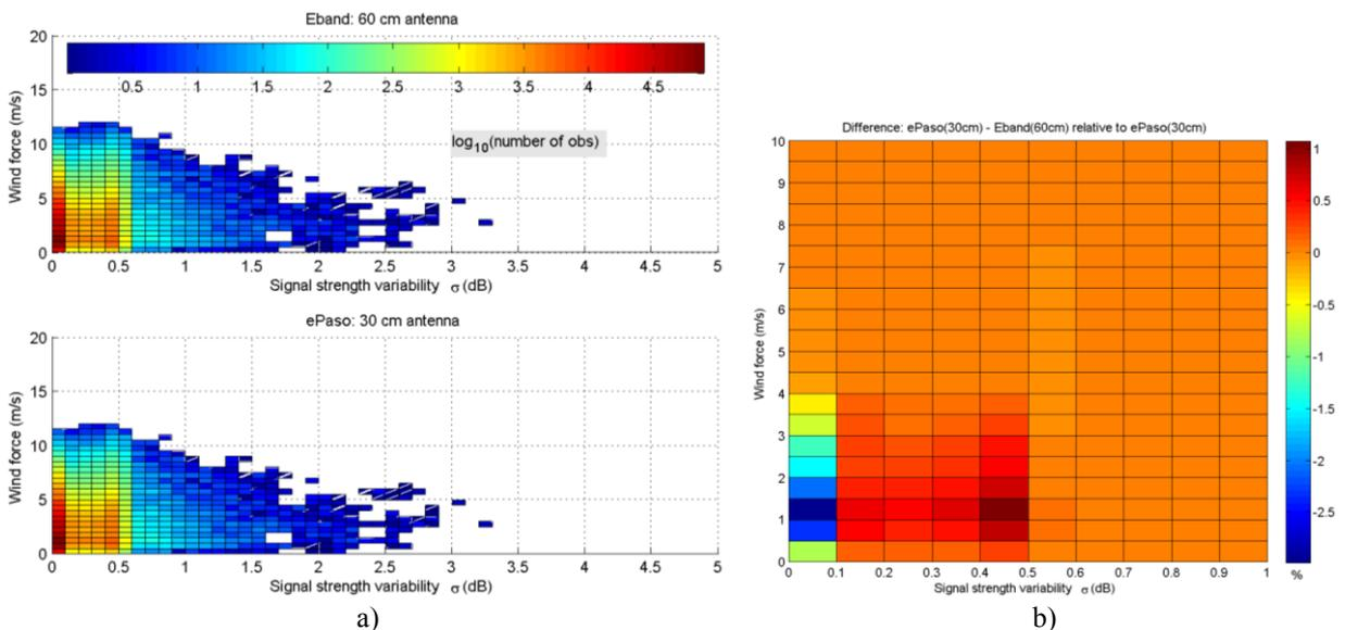
Figure 3. Signal variability (dB) per minute wind force a) comparing the links 60 cm and 30 cm reflector antenna diameters, and b) the difference (%) between to wider beam and the narrower beam relative to the wider beam.
