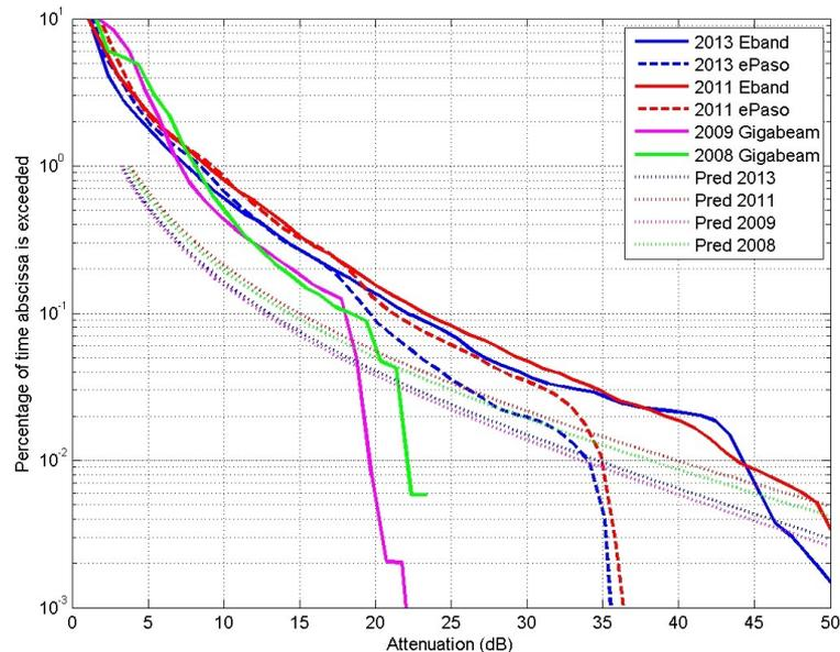
Figure 1. Measured precipitation attenuation distributions for 2008, 2009, 2011, and 2013 compared with yearly predictions using local rainfall rate data.
