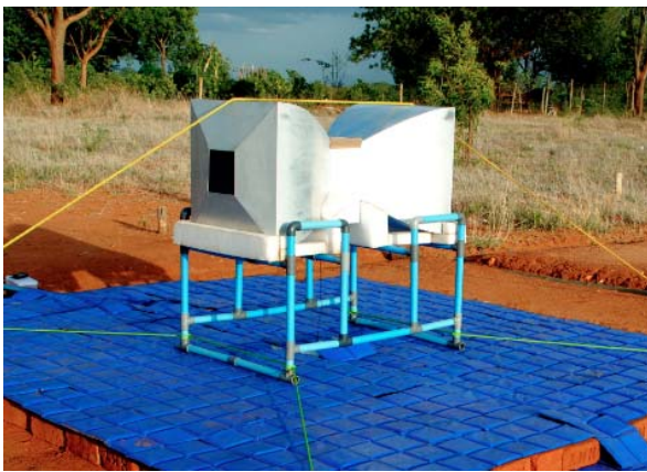
Fig. 1. The SARAS fat dipole antenna in the field. Analog receiver is partly in a compact unit between the arms of the dipole and partly below the ferrite tiles covering the ground, RF over fiber runs from the dipole 100 m away to a remote shed that houses further amplifiers and filters that define the band and the digital spectrometer.
