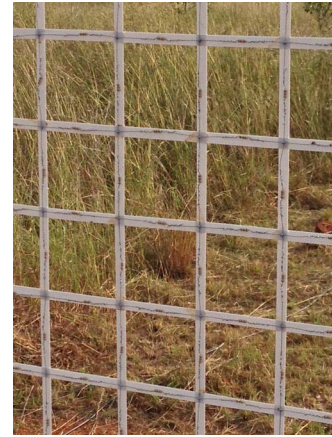
Fig. 4. Prototype resistive sheet built as a soldered square grid of resistors for field measurement of transmission and reflection coefficients.
