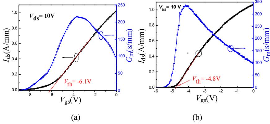
Figure 3: Transfer characteristics of the AlGaIn/GaN HEMTs on sapphire(a) and SiC substrate(b).
