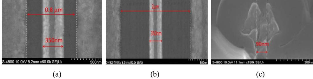
Figure 1: SEM image of AlGa<sub>N</sub>/Ga<sub>N</sub> HEMTs on sapphire (a), SiC substrate (b) and the 90-nm T-shaped gate (c).
