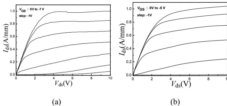
Figure 2: DC Output characteristics of the AlGa<sub>N</sub>/Ga<sub>N</sub> HEMTs on sapphire (a) and SiC substrate (b).
