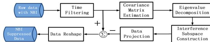
Fig. 2. Flowchart of the Eigensubspace-based NBI suppression method for a single pulse.
