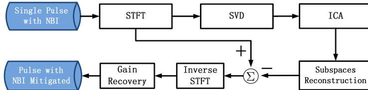
Fig. 4. Flowchart of the ISA-based NBI suppression method for a single pulse.
