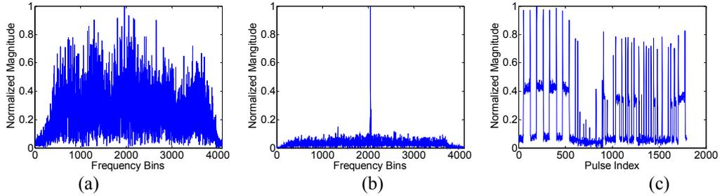
Fig. 1. Comparison between the spectrum of measured pulses (a) without NBI and (b) with NBI. (c) Variation of the normalized amplitude with pulses for a certain range bin.
