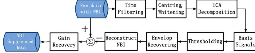
Fig. 3. Flowchart of the ICA-based NBI suppression method for a single pulse.
