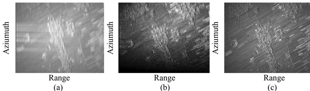
Fig. 5. Imaging results of the measured data. (a) Image of the raw data without NBI mitigation. (b) Image after frequency domain notched filtering. (c) Image using the proposed methods.
