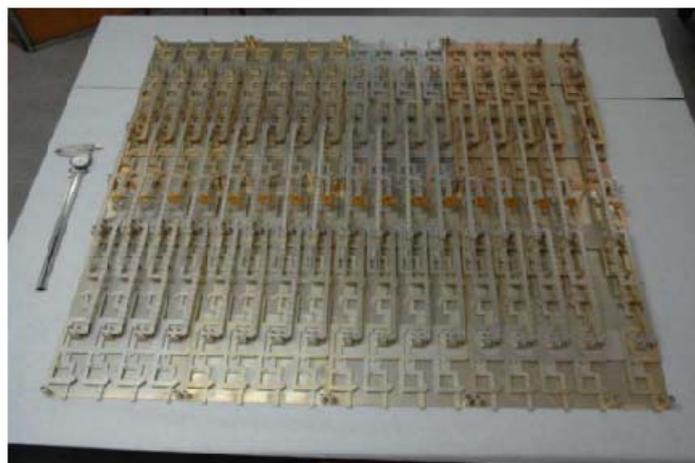
Fig. 2 Demonstration array with 16 receive sticks and one transmit stick
