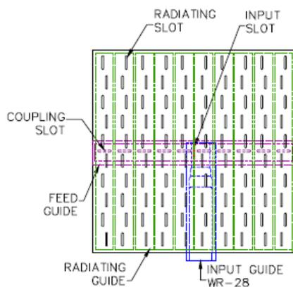
Fig. 3 Geometry of a sub-array with alternating offsets in adjacent waveguides
