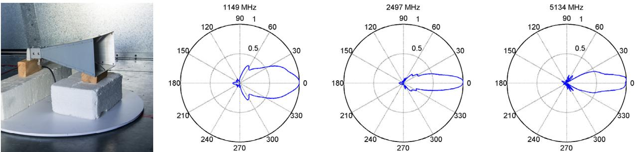
**Figure 2: Turntable and horn antenna in GTEM 1250 with radiation patterns in H-plane**
