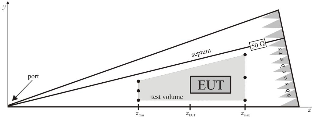
**Figure 1: Side view of a GTEM cell with the test volume and the calibration points at  $z_{\min}$  and  $z_{\max}$**
