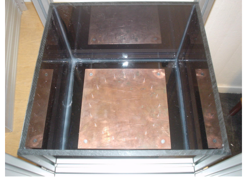
Figure 2: Photo of the imaging system. The 20 monopole antennas are mounted on a copper ground plane.
