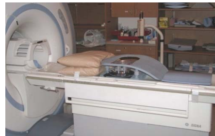
Figure 1: Photograph of the patient support platform positioned on top of a standard MRI couch.
