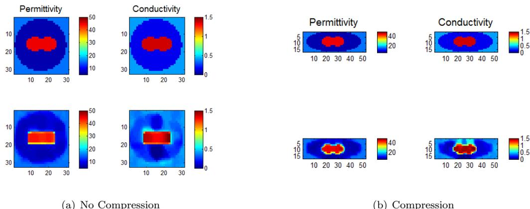
Figure 2: Reconstruction results for the object with and without compression after 3000 iteration steps. The permittivity (columns 1 and 3) and conductivity (columns 2 and 4) of the original (top) and reconstructed object (bottom). The axes are indexed by pixel number.
