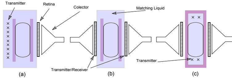
Figure 1: Different configurations for a planar MT system. (a) Single retina camera. (b) Double retina Camera. (c) Waveguide.
