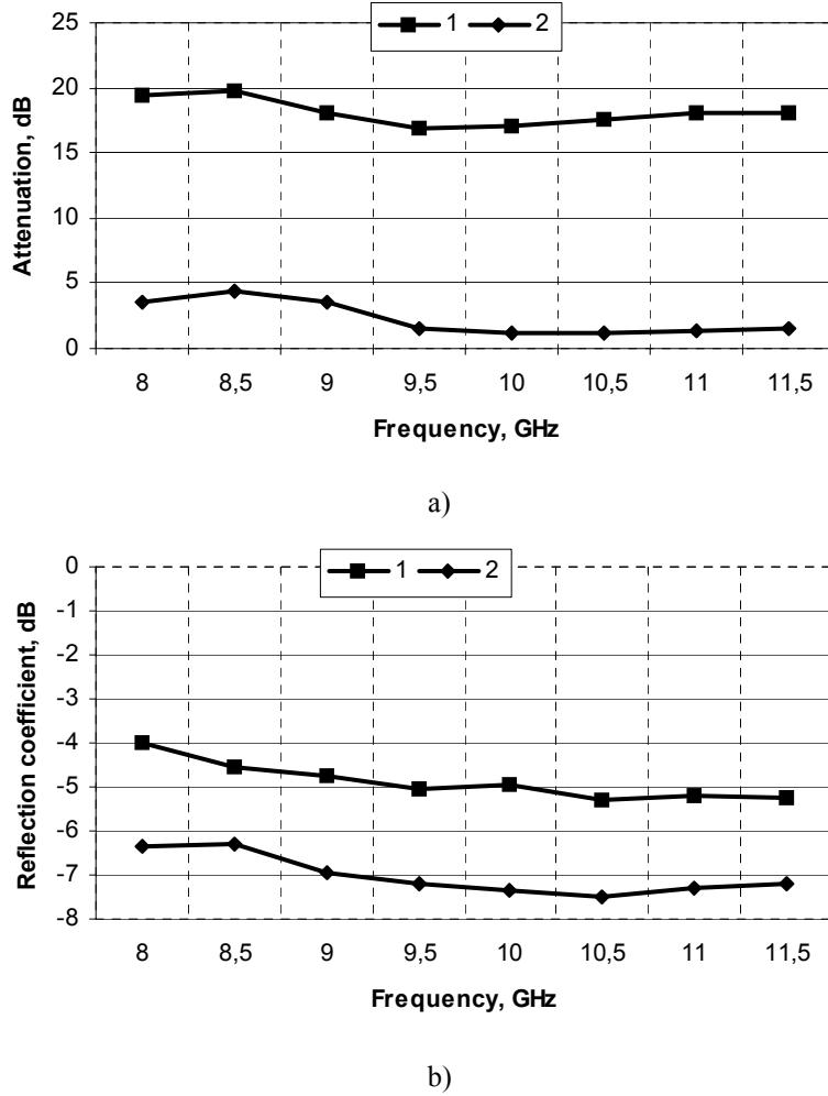
Figure 1 – Attenuation (a) and reflection (b) of electromagnetic emission by composite materials in the frequency ranges 8...11,5 GHz: 1 – sample with magnetic inclusions; 2 – sample without magnetic inclusions.
