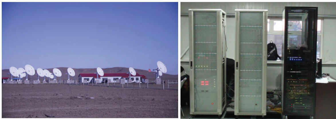
Figure 3 (left) CSRH-I central part antennas; (right) analogous receivers and monitor subsystems.
