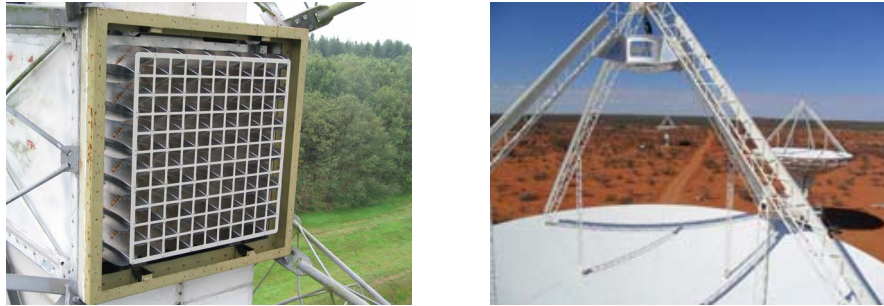
Figure 1. An 121-element APERTIF PAF installed in the WSRT (left) and the first ASKAP dishes (right)
