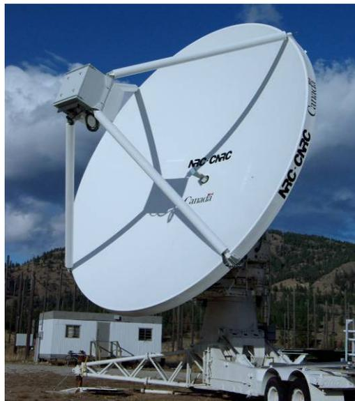
Figure 1: The MkII 10m one piece composite radio reflector
