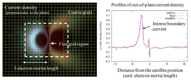
Contour map of out-of-plane current density (left panel) and its profile in the equatorial direction (right panel). Fine grids are adaptively generated at the boundary current layer where the variation of magnetic fields is large.
