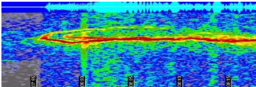
Figure 1: Start of morning F layer single hop propagation
