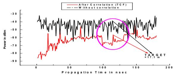
Fig. 8: Clutter rejection using Auto-correlation with Transmitted barker Code
