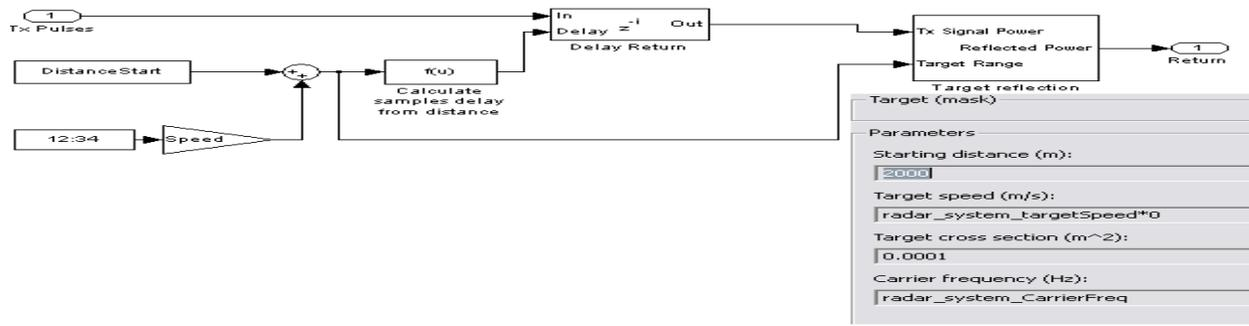
Fig. 4: Single Target Model
