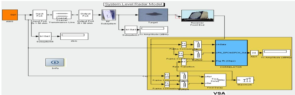
Fig. 1: The END-TO-END Simulation of the spread spectrum radar
