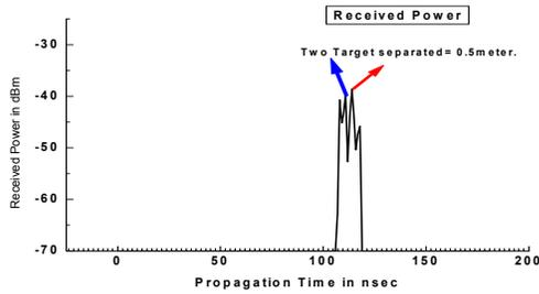
Fig.7: Range estimation for double targets ( $R_1= 16.55\text{m}$ ,  $R_2= 17.1\text{m}$ ).
