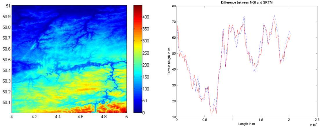
Fig. 2: left: terrain of Belgium (x-axis= $^{\circ}$  East; y-axis= $^{\circ}$  North); right: comparison between the data provided by the Belgian National Geographic institute and the SRTM (one random cut over about 20 km).
