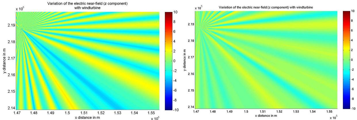
Fig. 6: Worst case deviations (left: 118 MHz, nacelle WE, blades 40°; right 156.3 MHz, nacelle NS, blades 40°).
