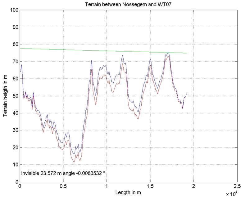
Fig. 3: determination of the non-illuminated part taking into account terrain, showing that the lowest 23.6 m are not visible from the RF source located at 0 on a 14 m high tower.
