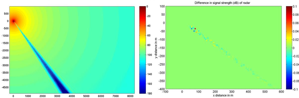
Fig. 4: difference between the radar considered as a point source and a linear equidistant array.
