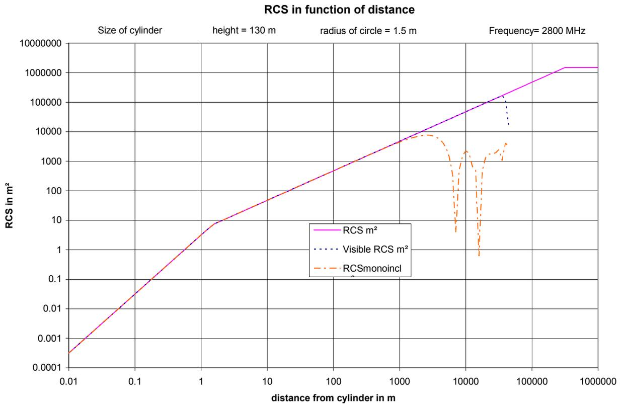
Fig. 5: Near-field monostatic radar cross section of a turbine tower.
